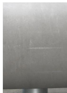
Non-optimal coating (steel group E)
