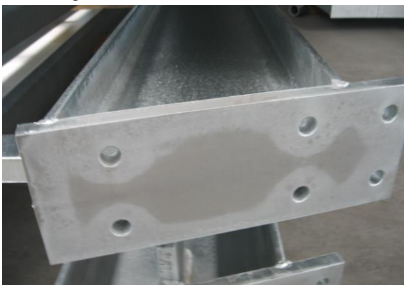
Heat stains because of thick material
