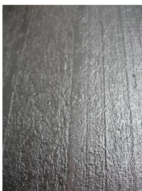
Non-optimal coating (steel group B)
